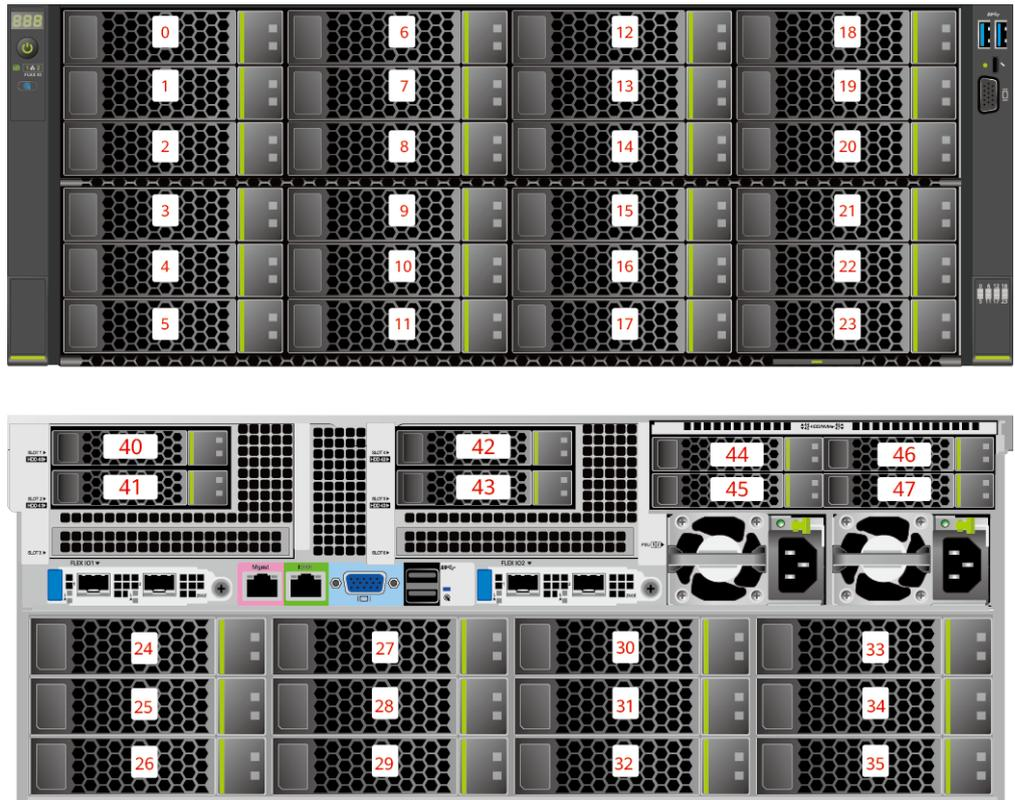
**Figure 5-18** Drive slot numbers (2.5" drives in I/O module 1 and 3.5" drives in I/O module 2)
