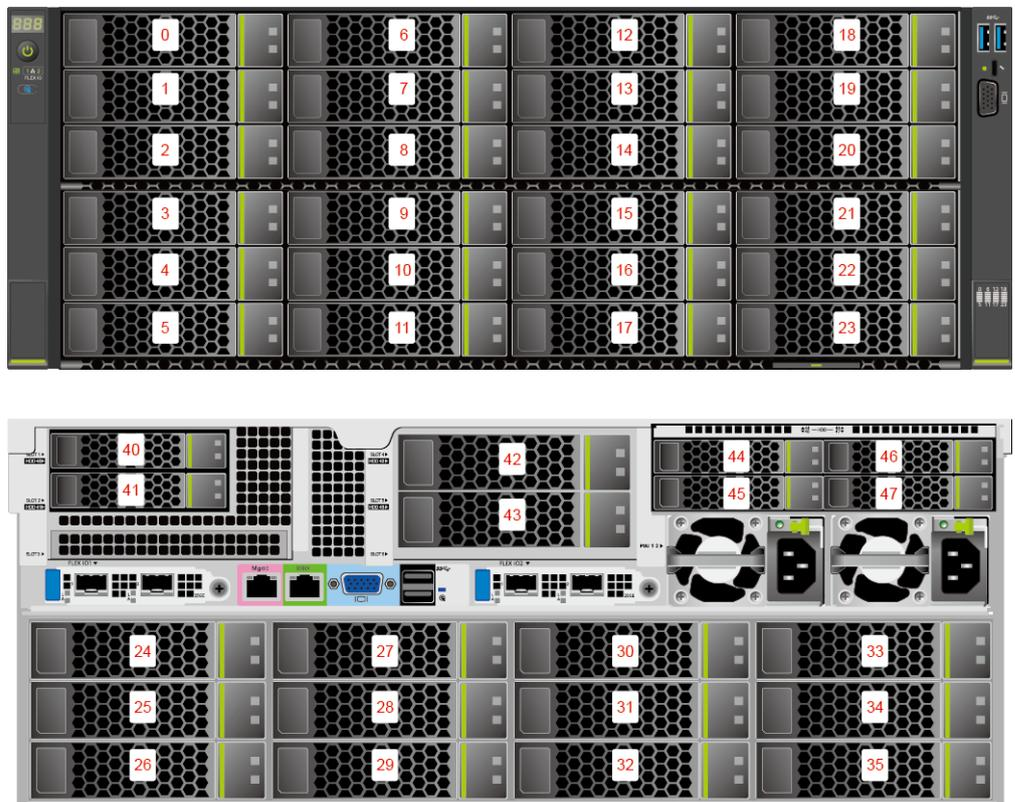
**Figure 5-19** Drive slot numbers (3.5" drives in I/O module 1 and 2.5" drives in I/O module 2)
