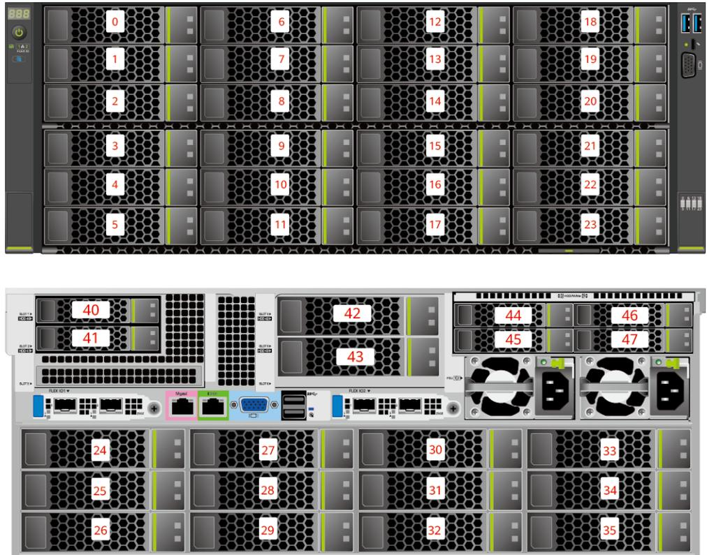
**Figure 5-27** Drive slot numbers (2.5" drives in I/O module 1 and I/O module 2)
