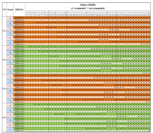
Figure 5-18 DDR4 memory installation guidelines (4 processors)
