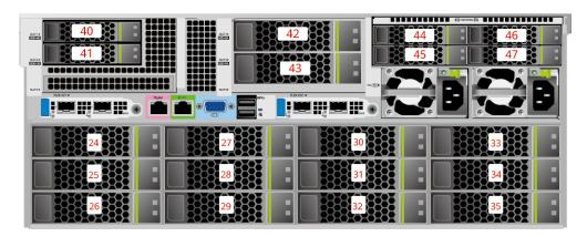
Figure 5-27 Drive slot numbers (2.5" drives in I/O module 1 and I/O module 2)
