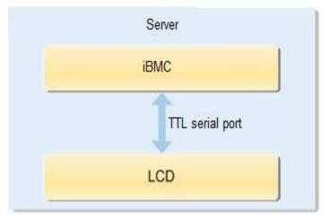
Figure 5-49 LCD subsystem working principle
