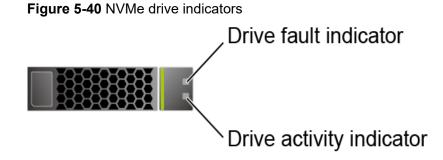
• If the VMD function is enabled and the latest VMD driver is installed, the NVMe drives support surprise hot swap.
